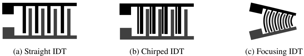
Figure 2.6: Examples of IDT configurations. The illustrations were created by the author based on the configurations described by Song et al. [2].
