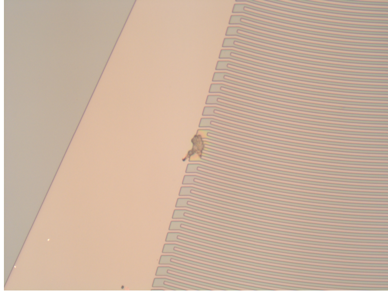
Figure 4.14: Residue or defect observed near the edge of the IDT fingers before metal evaporation.
